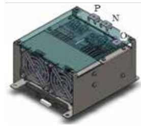
Example hardware SiC Switching pole (Chopper-cell module) 700V/30A
